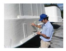
Once the swimming pool is manufactured we use an ultrasonic thickness tester to ensure that the materials have been applied in the correct thicknesses. Further, to ensure correct cure on our product we use a barcol hardness testing device to ensure the resins and gelcoats have correctly cured.
