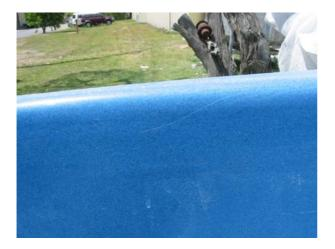
• Using a die grinder grind along the crack down to the thickness of the original gelcoat.
