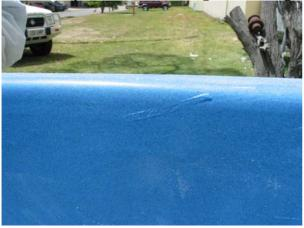
• Once the gelcoat has gone hard, place some acetone on a rag and rub the repair to remove any stickiness.
