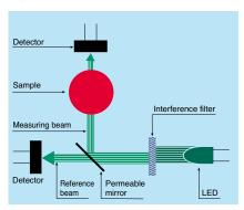
Twin light-beam technology guarantees optimum precision with PoolDirect photometers.
