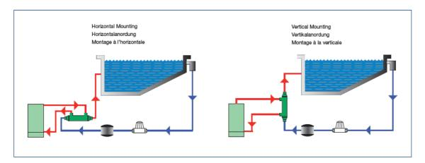
The heat exchanger may be damaged by chemicals. Dosing systems must be fitted downstream from the heat exchanger incorporating a non return valve. If chemicals are used, gases must be prevented from entering the heat exchanger when the filtration system is not in use.
