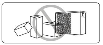
1.4.4. Don't put anything into inlet or outlet, or the efficiency of the heat pump will be reduced or even stopped.
