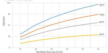
kW Heat Transfer - EC160-5113-5 Pool water flow 250 l/min at 28°C
