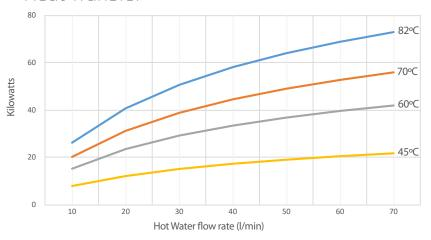
kW Heat Transfer - EC120-5113-3 Pool water flow 250 l/min at 28°C
