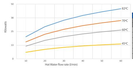
kW Heat Transfer - EC100-5113-2 Pool water flow 250 l/min at 28°C
