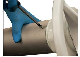
**6.** Secure the gearbox end oss to the reel tube through the drilled holes using the two supplied screws with a cross/ pozi head screwdriver.
