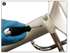
**1.** Undo the two slidelock end boss retaining screws.
