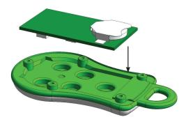
Put the electronic card back in its housing.
