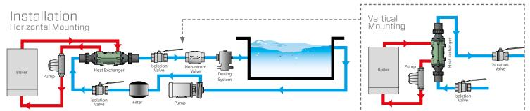
If an automatic dosing system is added, it must be installed after the heat exchanger on the return to the pool.
