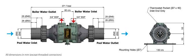
Max. Operating Туре **Tube Material Typical Pool Maximum Pool Maximum Hot** Max. Operating Weight Pressure Pool Water Pressure Hot Water Capacity Water Flow Water Temp m³ gal m³∕h l/min ۰C bar bar psi psi EC80-5113-1C Cupro-nickel 8,800 9.0 150 110 230 40 6 87 6 87 EC80-5113-1S\* **Stainless Steel** 50 11,000 12.0 200 110 230 6 87 6 87 EC80-5113-1T Titanium 60 11,000 12.0 200 110 230 6 87 6 87
