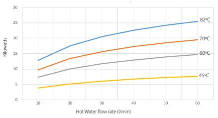
kW Heat Transfer - EC80-5113-1 Pool water flow 200 l/min at 28°C
