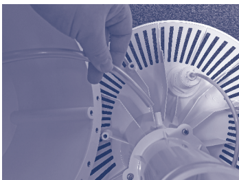
Fig 7: Connection of air supply tube from housing to faceplate.
