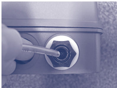
Fig 10: Air control tube connection to electro-pneumatic control box.
